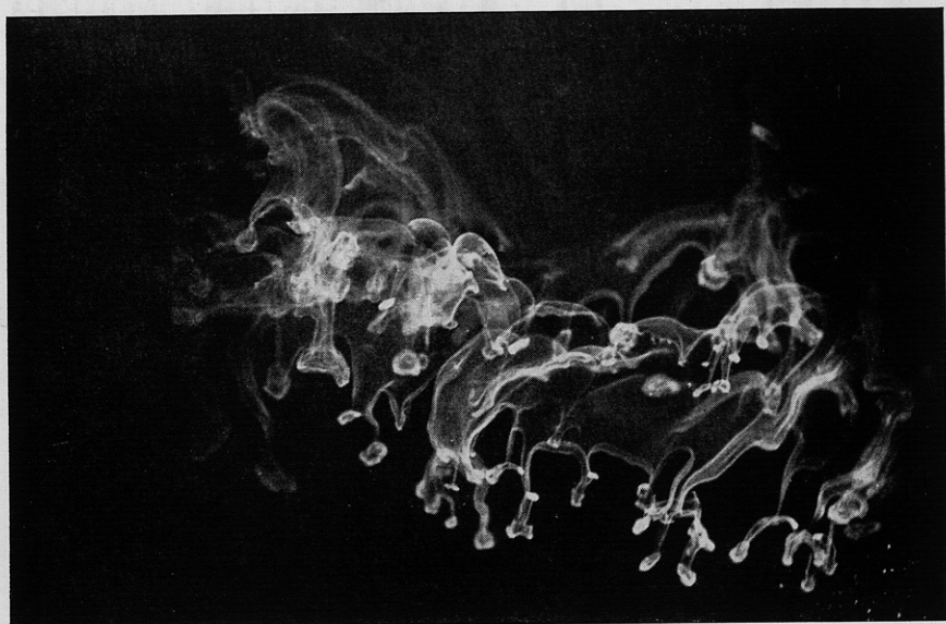
FIG. 8. Trail of ice crystals produced in cold chamber by seeding with needle cooled below -39^{\circ}\text{C} .
